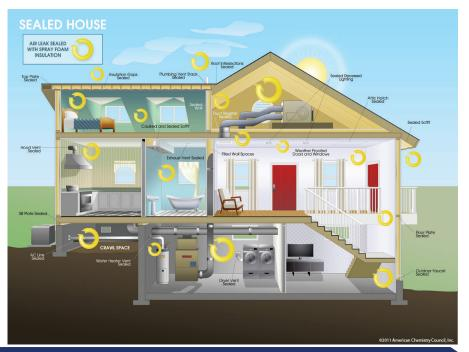
Some common spots for air leaks that can be sealed with spray foam include the area behind knee walls, attic hatches, wiring holes, plumbing vents, open soffits, recessed lights, furnace flue or duct chaseways, basement rim joists, windows and doors.<sup>3</sup>
